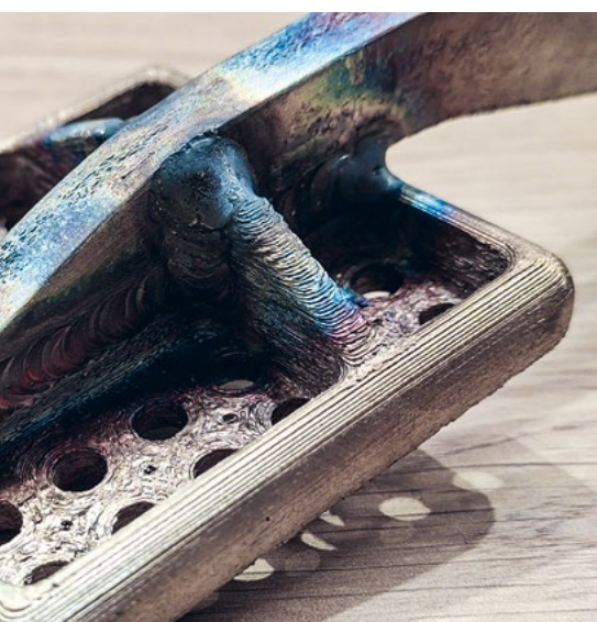
Prototype Land Rover brake peddle printed in 4 sections with Metal Paste Deposition in 17-4PH Stainless Steel and TIG welded together to optimise production cost and time.
