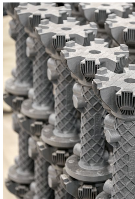
Hydrogen compressor developed by Bosch in cooperation with Nikon. The component, which is made from AlSi10Mg, was produced in 48 hours in a NXG XII 600 and combines lightweight construction with various in-built features, designed to improve overall performance.
