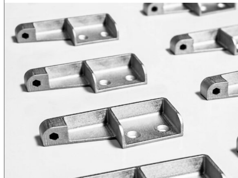
Photo left page: The Ford development team uses desktop SLA 3D Printing to manufacture various prototypes.
