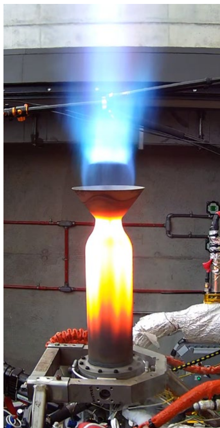
Intuitive Machines printed this rocket nozzle component for the IM-1 mission to the moon
