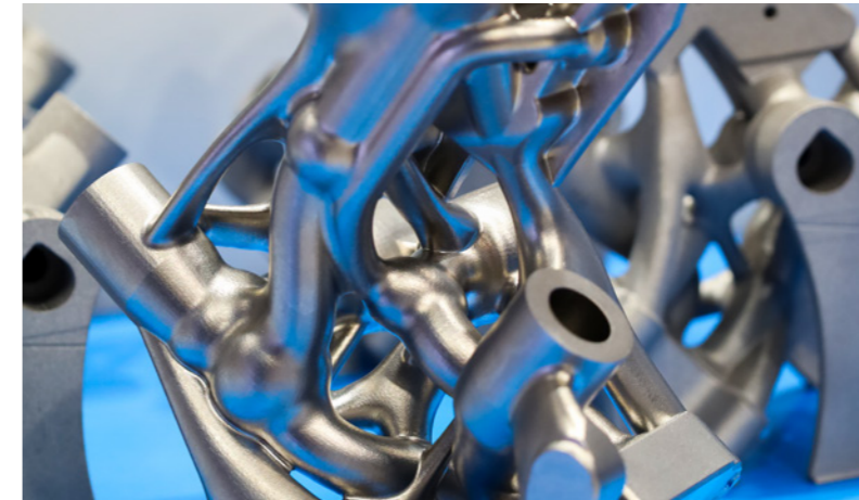
At left: A manifold made of Ti6Al4V that was developed by Airbus and manufactured on an M2 Series 5 machine from Colibrium Additive At right: An RL 10 engine from L3 Harris
