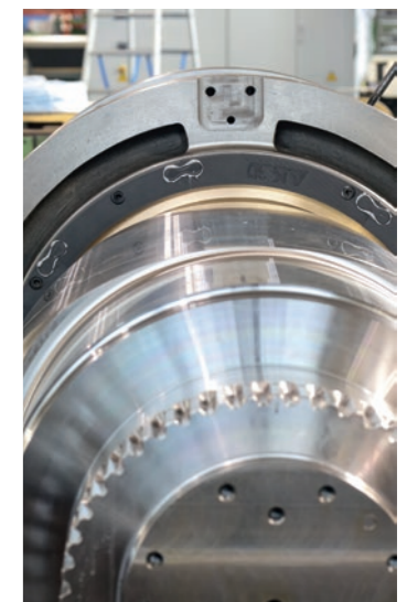
An eccentric shaft with oil drainage rings
