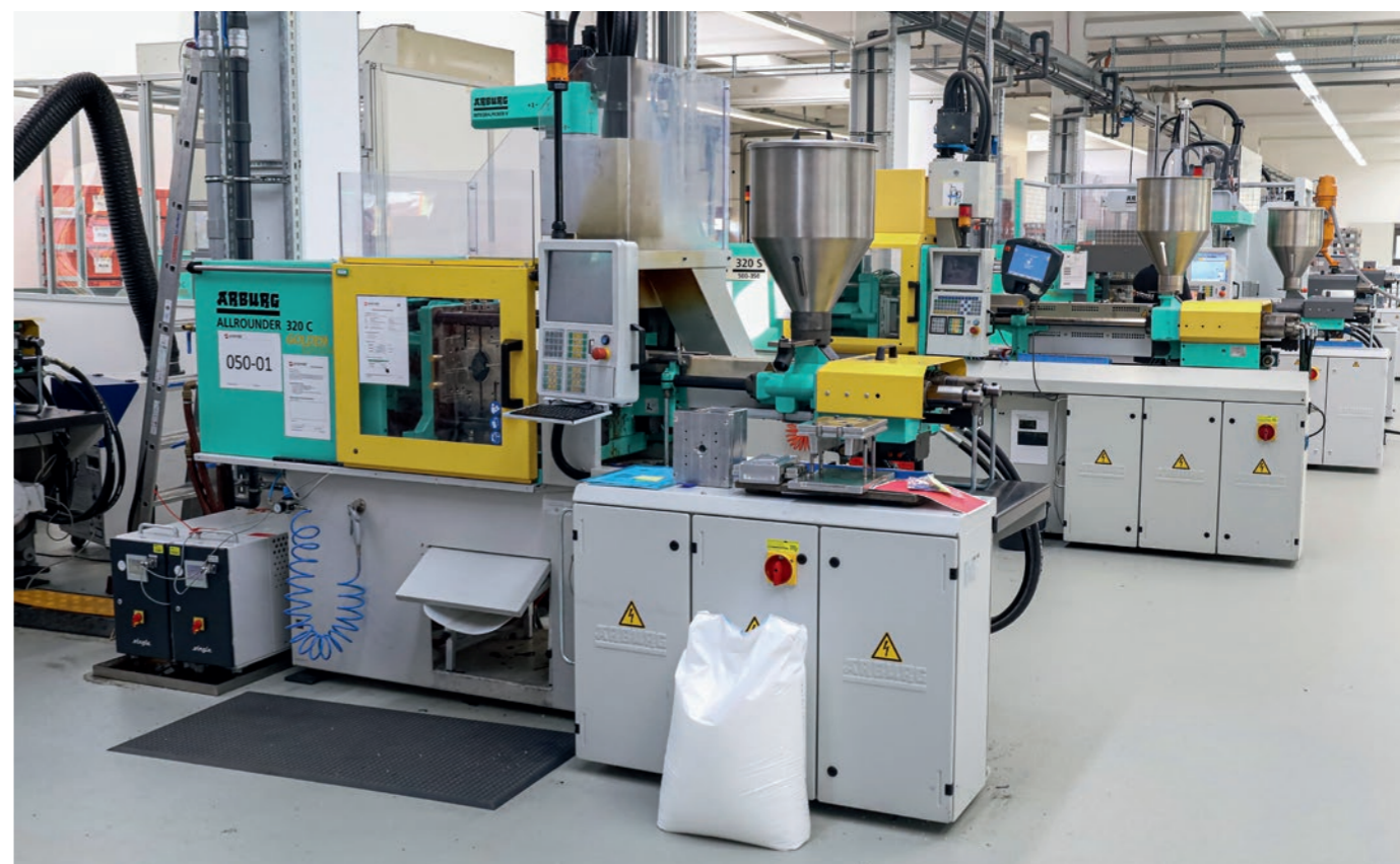
Left: Thomas Schönbucher and Felix Parsch in Priomold's AM department Below: The core of Priomold's business: an array of injection molding machines producing prototypes and small series
