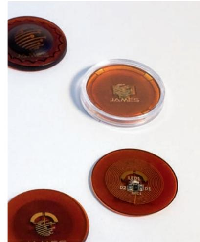
*Top photo:* The J.A.M.E.S Coin is a near-field communication tag that demonstrates a way to print antenna coils and free-formed plate capacitors under the strictest space limitations
