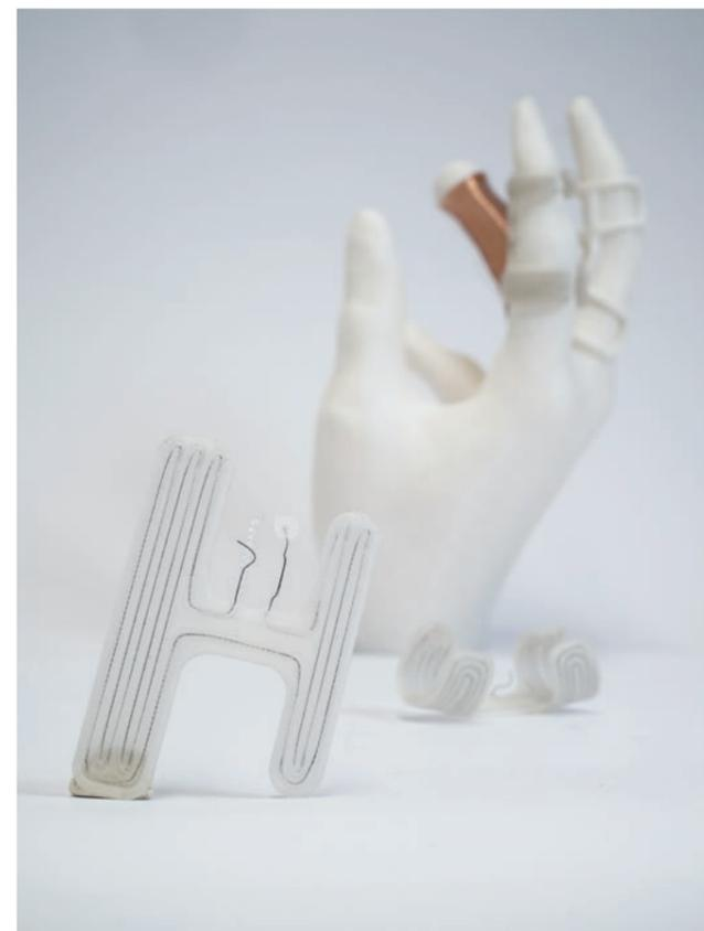
Various electronic applications from Fraunhofer IWU: finger orthotics manufactured using WEAM (left); 200-µm copper wire on 100-µm film with printed-on structural components (p. 13, top); and a WEAM printer head with integrated process monitoring (p. 13, middle)
