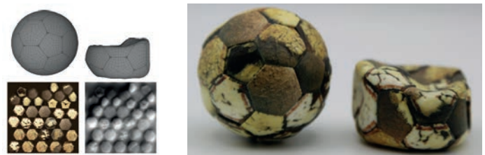
Input Figure 2: A model comprised of disjoint mesh patches, a displacement map, and a color texture map (left), and the resulting print using displaced signed distance fields (right). The total geometry storage is only 2MB.
