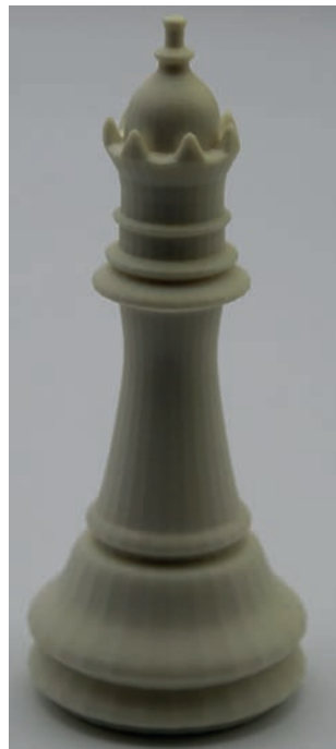
Input Figure 2: A model comprised of disjoint mesh patches, a displacement map, and a color texture map (left), and the resulting print using displaced signed distance fields (right). The total geometry storage is only 2MB.
