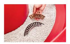
tor bed. The vibration of the trough produces relative motion between the workpiece and the rotary vibrators, which in turn results in a smooth, consistent surface. Christoph Cruse, director of sales at Walther Trowal, describes the TRT 83/87 as a machine suitable for those just getting started in AM.
